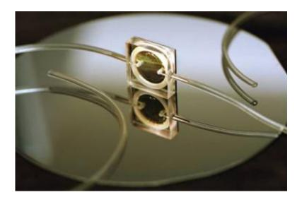
Single cells can flow through this nanoscale biocavity laser, enabling malignant cells to be differentiated from normal cells. Courtesy of Sandia National Laboratory.
