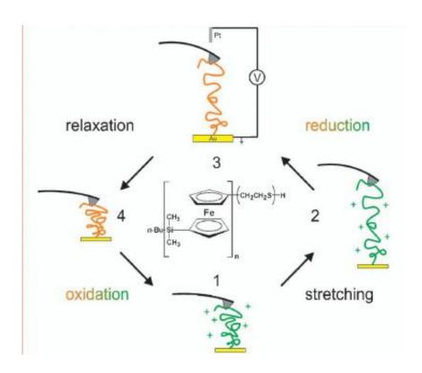
The cycle of oxidation and reduction, causing soft/hard transitions within the molecule. The associated stretching and shrinking gives the mechanical energy. The forces are monitored by the tip of an Atomic Force Microscope, on top of the molecule. The bottom of the chain is fixed on a gold surface.
