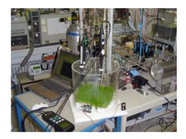
A plant chamber used to investigate methane formation in plants -- in this example, in ryegrass (Lolium perenne). Image: Max Planck Institute for Nuclear Physics.
