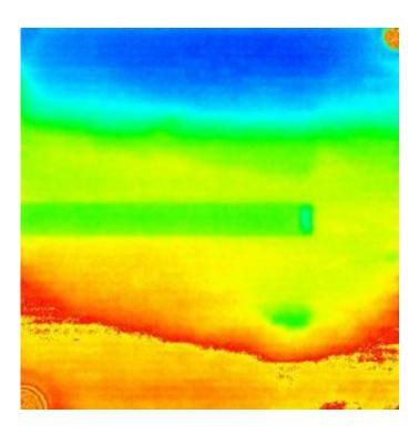
Liquid water content of an operating PEM fuel cell. Red color is more water, blue is less.
