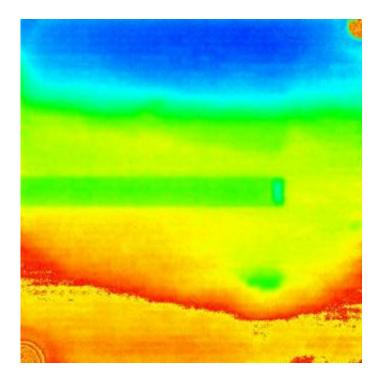
Liquid water content of an operating PEM fuel cell. Red color is more water, blue is less.
