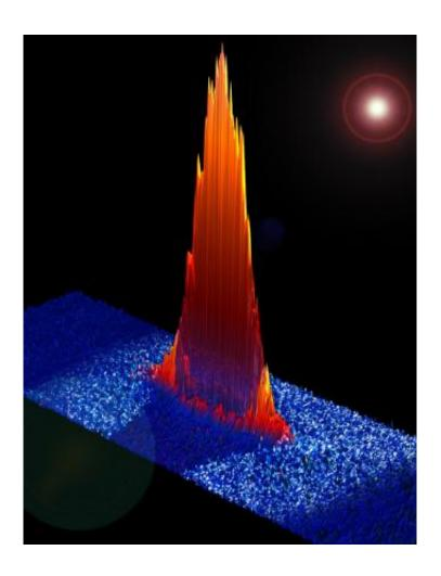
This is a 3-dimensional projection of an image of a phase separated atomic cloud. The tall central (semi-transparent) region consists of paired fermionic 6 Li atoms, and is believed to be a superfluid. The shorter (opaque) peaks on either side, as well as the faint ring around the bottom, are unpaired atoms which have been expelled from the paired central region. The light in the background is a representation of the probe laser beam used to image this cloud.
