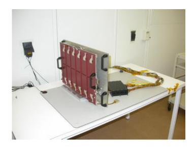
Image: All three components of the SDC assembled and ready to be put into the New Horizons spacecraft. If you will notice, the dust detector itself is protected from dust hitting it before it is supposed to.
