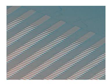
The next wave in electronics could be wavy electronics. Researchers at the University of Illinois at Urbana-Champaign have developed a fully stretchable form of single-crystal silicon with micronsized, wave-like geometries that can be used to build high-performance electronic devices on rubber substrates.
