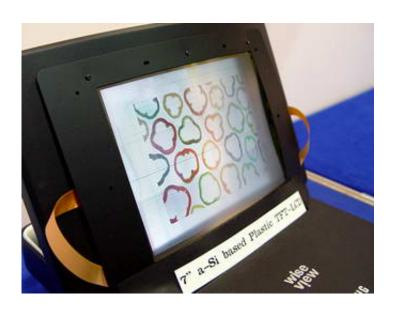
Samsung Electronics announced that it has developed the world's largest transmissive TFT LCD (thin-film transistor, liquid crystal display), with sufficiently high resolution to display digital television content. The seven-inch, 640x480 (VGA-standard) flexible display uses a transparent plastic substrate that is thinner, lighter and more durable than the conventional LCD glass panels used today.
