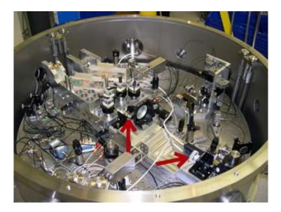
A new laser-based method for measuring millimeter distances more accurately than ever before--with an uncertainty of 10 picometers (trillionths of a meter)--has been developed and demonstrated by a physicist at the National Institute of Standards and Technology. This is akin to measuring the distance from New York to Los Angeles with an uncertainty of just 1 millimeter. The technique may have applications in nanotechnology, remote sensing and industries such as semiconductor fabrication.
