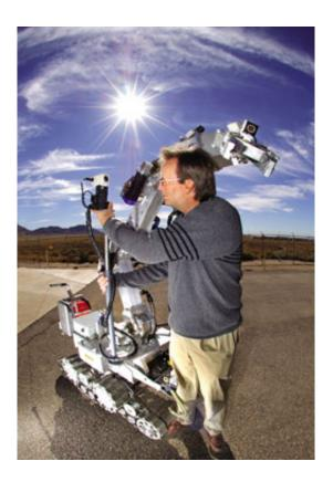
A Sandia National Laboratories robot recently withstood enough radiation to kill 40 men in freeing a stuck radiation source -- the size of a restaurant salt shaker -- at a White Sands Missile Range lab so that the cylinder could be safely returned to its insulated base.
