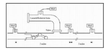
Detecting leaks and conducting maintenance in America's aging network of natural gas pipelines will eventually be a job for wireless robots, according to researchers at the University of Missouri-Rolla.
