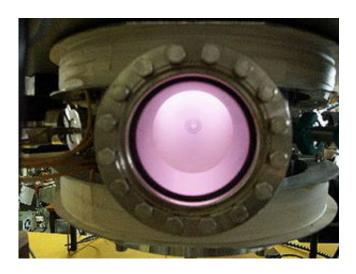
ESA has confirmed the principle of a new space thruster that may ultimately give much more thrust than today's electric propulsion techniques. The concept is an ingenious one, inspired by the northern and southern aurorae, the glows in the sky that signal increased solar activity.
