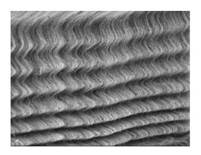
Carbon nanotubes have enticed researchers since their discovery in 1991, offering an impressive combination of high strength and low weight. Now a new study suggests that they also act like supercompressible springs, opening the door to foam-like materials for just about any application where strength and flexibility are needed, from disposable coffee cups to the exterior of the space shuttle.
