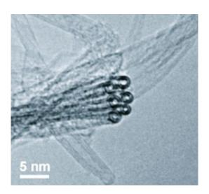
Image: An electron microscope image shows a bundle of nanotubes.
