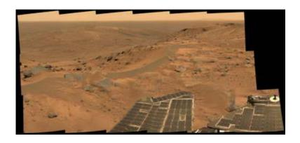
"We followed a circuitous path uphill, using the higher, uneven terrain to tilt the solar panels toward the Sun, keep the communications antenna facing Earth, and avoid rocks along the way," said rover driver Chris Leger at NASA's Jet Propulsion Laboratory.
