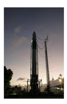
Space Exploration Corp. (SpaceX) launch scrubbed Saturday because of problems with liquid oxygen (LOX) fill tank. The reason for the delay was that an auxiliary liquid oxygen fill tank had a manual vent valve incorrectly set to vent. The time it took to correct the problem resulted in significant LOX boiloff and loss of helium, and it was the latter that
