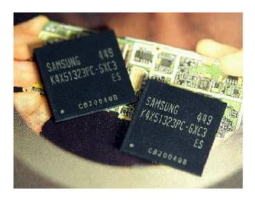
Samsung Electronics announced that it has started to mass produce 512Mb DRAM (dynamic random access memory) for mobile products, using 90nm circuitry. This marks the first time that 512Mb mobile DRAM will be available anywhere and the first time that nano-scale process technology will be used in the production of any mobile DRAM.
