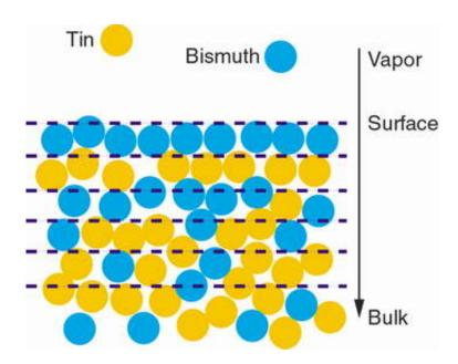
With the help of the world's most brilliant hard X-ray beams at the Advanced Photon Source, scientists have seen for the first time metal atoms near the surface of a liquid alloy arrange themselves in alternating layers one atom thick.
