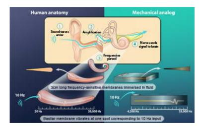
Researchers at the University of Michigan are developing a mechanical cochlea, a device that functions much like its human counterpart in the ear. Yet, because it is composed of micromachined parts and integrated circuits, the apparatus should be inexpensive to manufacture and could potentially capture a range of frequencies well beyond those of human hearing.
