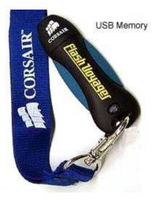
It's predicted in the long run these devices will even replace your computer's hard drive. Two factors are currently blocking this change: First, they cost more per GB – about 10 times more at the writing of this article. Second, they have a limited number of erase operations that can be preformed depending on the type – anywhere from low of 10,000 to a high of 1,000,000. So they do wear out – but only after long, hard use.
