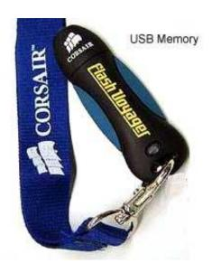
It's predicted in the long run these devices will even replace your computer's hard drive. Two factors are currently blocking this change: First, they cost more per GB – about 10 times more at the writing of this article. Second, they have a limited number of erase operations that can be preformed depending on the type – anywhere from low of 10,000 to a high of 1,000,000. So they do wear out – but only after long, hard use.
