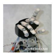
A highly dexterous, bio-inspired artificial hand and sensory system that could provide patients with active feeling, is being developed by a European project.
