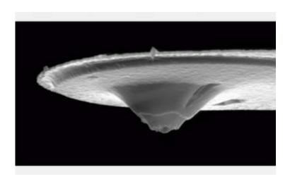
Image: This scanning electron micrograph shows the new nanofountainprobe dispensing tip. Credit: © 2005 Horacio D. Espinosa
