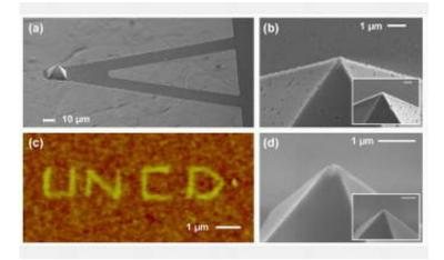
Image: This slide highlights the ultra-nano-crystalline diamond (UNCD) atomic force microscope (AFM)cantilever. (a) This is a scanning-electron micrograph of a UNCD cantilever with a tip. (b) This is a scanning electron micrograph of a UNCD tip after one hour of scanning on a diamond substrate. Inset shows the tip before the scanning. (c) This is a frictional AFM image of an alkanethiol monolayer patterned onto a gold substrate with a UNCD tip. Researchers used the same tip for patterning
