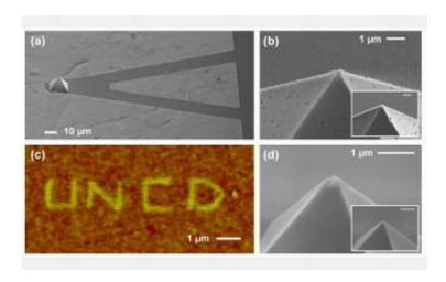
Image: This slide highlights the ultra-nano-crystalline diamond (UNCD) atomic force microscope (AFM)cantilever. (a) This is a scanning-electron micrograph of a UNCD cantilever with a tip. (b) This is a scanning electron micrograph of a UNCD tip after one hour of scanning on a diamond substrate. Inset shows the tip before the scanning. (c) This is a frictional AFM image of an alkanethiol monolayer patterned onto a gold substrate with a UNCD tip. Researchers used the same tip for patterning
