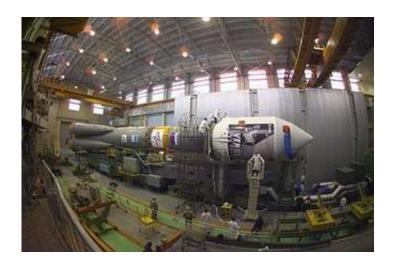
Following the announcement of the Venus Express launch delay due to particulate contamination found in the launcher fairing where the spacecraft was installed, ESA staff and industry teams have started an inspection of the spacecraft. This recovery 'investigation procedure' has so far revealed a spacecraft in good status.
