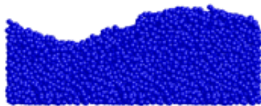
Growth simulation: deposition of 4000 carbon atoms on a rough substrate (Brenner)
