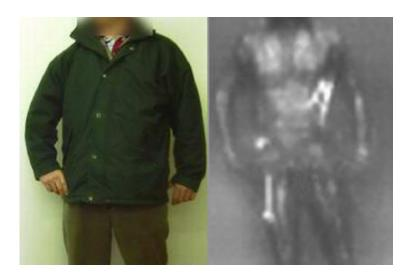
Metal detectors currently used for screening aircraft passengers could soon be supplanted by novel millimetre-wave cameras, able to detect even non-metallic concealed objects. The new system, named after a Brazilian bat, is based on technology developed for ESA spacecraft. Tadar is being demonstrated at this week's Inter Airport Europe Exhibition in Munich.
