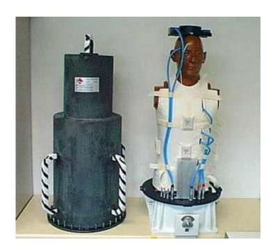
A phantom, which was outside the International Space Station for a year and a half, is now inside with the ISS crew. However this is no ghost story but a serious set of scientific experiments to monitor radiation levels inside and outside the ISS.
