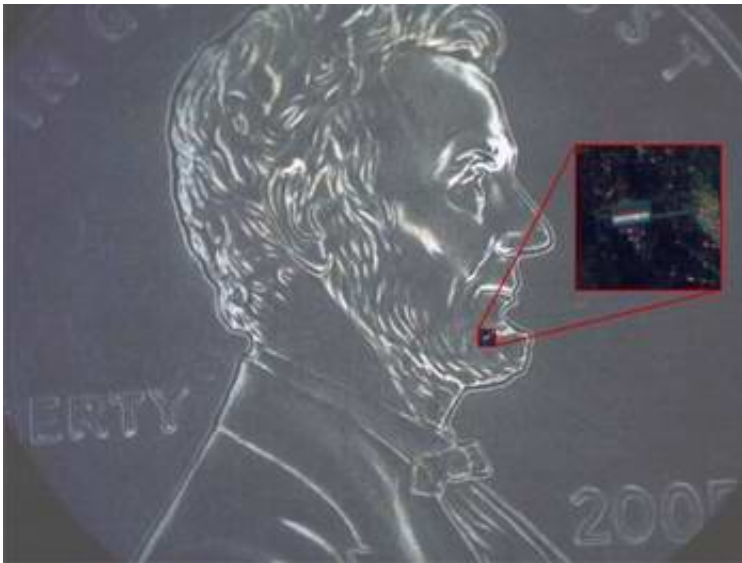
The microrobot on a penny. (Courtesy Donald Laboratory)
