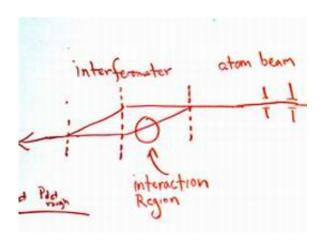
This simple sketch shows the placement of diffraction gratings - represented by the vertical dashed lines - that split and recombine atom waves. The gratings are about a meter apart.
