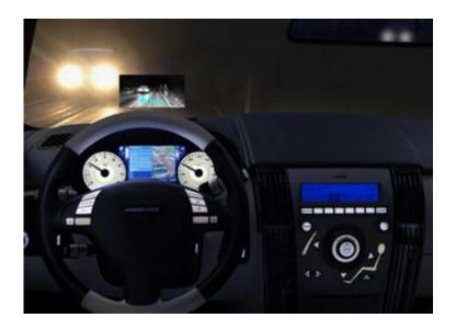
At the International Motor Show (IAA) in Frankfurt, Siemens has introduced a night vision system that works with infrared technology. With this innovation, Siemens has also become the first automotive industry supplier to create a prototype of an electronic pedestrian marking system. One quarter of all serious traffic accidents take place in the evening or at night. And about one third of all traffic fatalities are the result of accidents during these hours.
