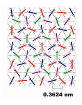
Image: Multi-colored arrows show the disordered array of magnetic spins of electrons within nickel gallium sulfide. The data were collected by precisely measuring the timing and change in direction of neutrons as they were passed through the material. Credit: S. Nakatsuji et al., Science, 9/9/2005
