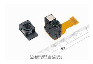
Sharp Corporation has developed two new 3-megapixel CCD camera modules intended for use in camera-equipped mobile phones. The two camera modules feature a built-in autofocus function and the new LZ0P3758 features, in addition, an all-internal optical zoom lens that is switchable between normal and 2X zoom, an industry first(\*1). Both models will be available in quantity beginning in September 2005.
