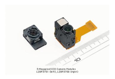
Sharp Corporation has developed two new 3-megapixel CCD camera modules intended for use in camera-equipped mobile phones. The two camera modules feature a built-in autofocus function and the new LZ0P3758 features, in addition, an all-internal optical zoom lens that is switchable between normal and 2X zoom, an industry first(\*1). Both models will be available in quantity beginning in September 2005.
