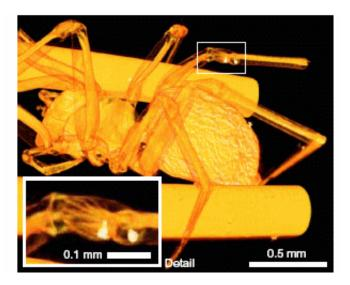
In a development that could help usher in a new kind of medical imaging for clinics and hospitals, researchers have demonstrated a practical x-ray device that provides 2- and 3-dimensional images of soft biological tissue with details that are ordinarily hard to discern with conventional x-ray imaging.
