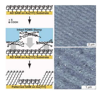
Scientists will announce next month a new technique called microdisplacement printing, which makes possible the highly precise placement of molecules during the fabrication of nanoscale components for electronic and sensing devices.
