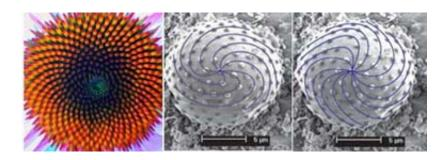
A coneflower showing 21x34 Fibonacci spirals at the primordium (left), and stress pattern on a flattened Ag core/SiO2 shell structure that can be grouped into 8 clockwise and 13 countclockwise spirals (center and right).
