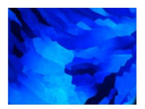
Liquid-crystal 'blue phases' can be just about any colour in the rainbow. This makes them potentially useful for all sorts of applications, from electrically switchable colour displays to light filters and lasers. But blue phases have a significant limitation: they exist over a very small range in temperature, typically no more than two degrees Celsius at most.
