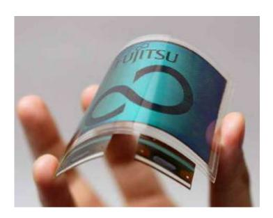
Fujitsu Laboratories Ltd., Fujitsu Frontech Limited, and Fujitsu Limited today announced their joint development of the world's first film substrate-based bendable color electronic paper with an image memory function. The new electronic paper features vivid color images that are unaffected even when the screen is bent, and features an image memory function that enables continuous display of the same image without the need for electricity.
