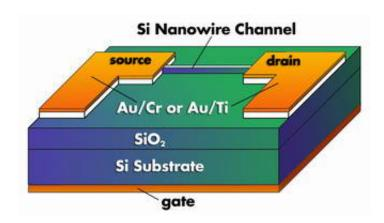
In an advance for nanoscale electronics, researchers at the National Institute of Standards and Technology (NIST) have demonstrated a new design for silicon nanowire transistors that both simplifies processing and allows the devices to be switched on and off more easily.
