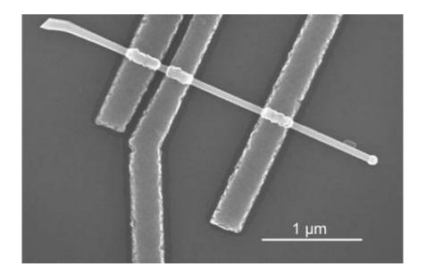
Image above: Scanning electron micrograph of one of the semiconductor nanowire devices. The nanowire is contacted by three superconducting aluminum contacts that induce the superconductivity in the nanowire. The device is fabricated on an oxidized doped silicon wafer that is used as a gate electrode in order to control the supercurrent. At the end of the wire the gold nanoparticle is clearly visible.
