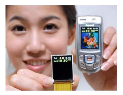
Samsung Electronics will introduce a new "section display" for mobile phones this fall. This display is divided into an indicator window and a main window and the low-power consumption quality of the new technology corrects the existing imperfections of external phone screens for an elegant, "always on," indicator display that requires virtually no power.
