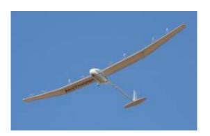
AeroVironment, a California-based company, says it has successfully completed a test flight of an aircraft powered by liquid hydrogen.
