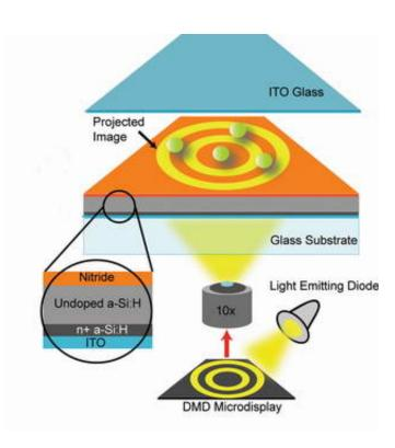
Rounding up wayward cells and particles on a microscope slide can be as difficult as corralling wild horses on the range, particularly if there's a need to separate a single individual from the group. But now, a new device developed by University of California, Berkeley, engineers, and dubbed an "optoelectronic tweezer," will enable researchers to easily manipulate large numbers of single cells and
