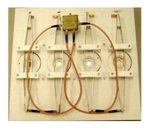
The electromagnetic system exposing four eye lenses to electromagnetic radiation Each vessel containing a lens, inserted between the two plates of the transmission line. The entire system is placed in an incubator maintaining constant temperature for the duration of exposure.
