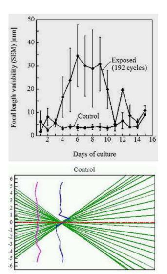
Good quality lens as demonstrated by the optical scanner. All rays passing Through the lens have similar focal length. The thick dashed line connects the points of the back vertex Distance for each ray passing through the lens. The thick solid line shows the relative intensity of each beam.
