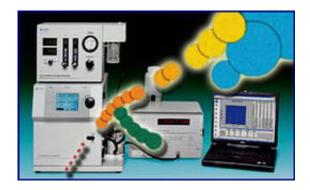
Ion Mobility Analysis makes use of a differential mobility analyzer and particle counter (left), an electrospray unit (center), and a computer to sort and count the numerous classes and subclasses of lipoprotein particles
