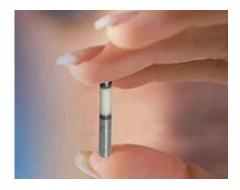
Argonne was involved in developing battery chemistry and materials for the microstimulator pictured above. The lithium-ion battery is the smallest cylindrical, rechargeable battery ever made.
