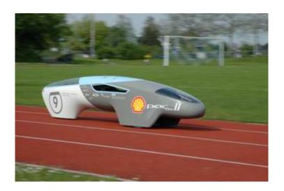
ETH Zurich set itself a goal to construct a vehicle that used as little fuel as possible and provided the highest possible fuel efficiency. So they gave the so-called PAC-Car a fuel cell that produces electrical energy from hydrogen and drives two electric motors. The only "emission" from PAC-Car is pure water. The car is lightweight, weighing in at only about 30 kilograms.
