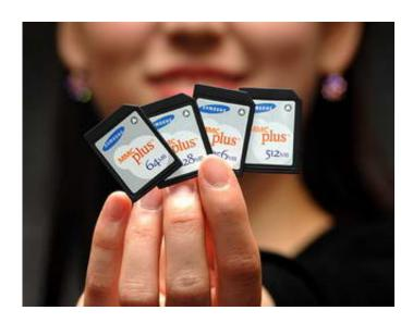
Samsung Electronics announced a major new commitment to the MultiMediaCard (MMC) market by initiating mass production of two new ultra-high-speed MultiMediaCards: MMC plus and MMC mobile. The new, ultra-fast MMCs are capable of transmitting data at 52MBytes per second, up to twenty times faster than existing MMCs, by supporting wider x4 and x8 bus widths.
