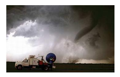
A new Doppler radar instrument that can scan tornadoes every five to 10 seconds is prowling the Great Plains this spring in search of its first close-up twister. Newly enhanced for season-long thunderstorm tracking, the radar promises the most complete picture to date of tornado evolution, allowing for better tornado prediction in the future.
