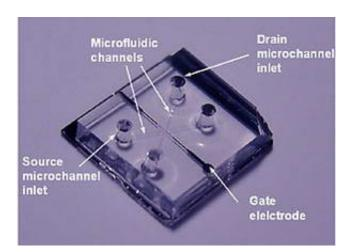
University of California, Berkeley, researchers have invented a variation on the standard electronic transistor, creating the first "nanofluidic" transistor that allows them to control the movement of ions through submicroscopic, water-filled channels.
