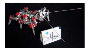
Many insects sense their way around their immediate surroundings by means of moving feelers. Now research scientists have applied this active spatial recognition of objects to create a new mechatronic type of sensor. It could soon be in use as an orientation aid for mobile robots.
