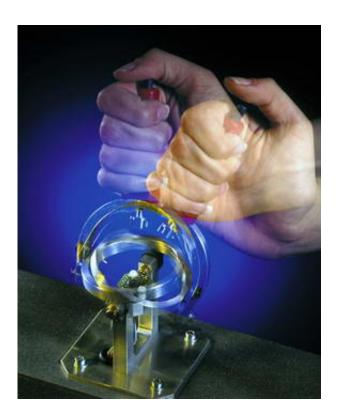
Gas and brake pedals have to react quickly and reliably if the occupants of the vehicle are not to be unnecessarily endangered. Engineers have developed a 3D magnetic sensor which digitally registers the pedal deflection by its angle. BMW is currently testing the system.
