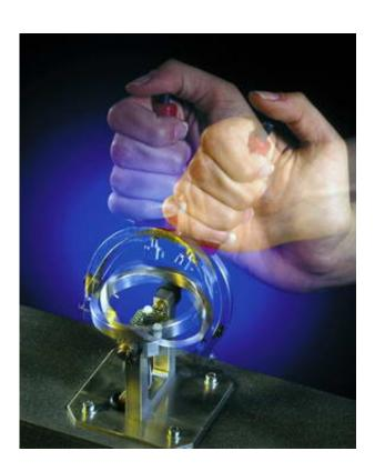
Gas and brake pedals have to react quickly and reliably if the occupants of the vehicle are not to be unnecessarily endangered. Engineers have developed a 3D magnetic sensor which digitally registers the pedal deflection by its angle. BMW is currently testing the system.
